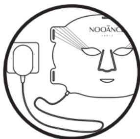
Connect the mask directly to the mains using the 2m cable supplied and the mains adapter (you will need to time your session manually).
